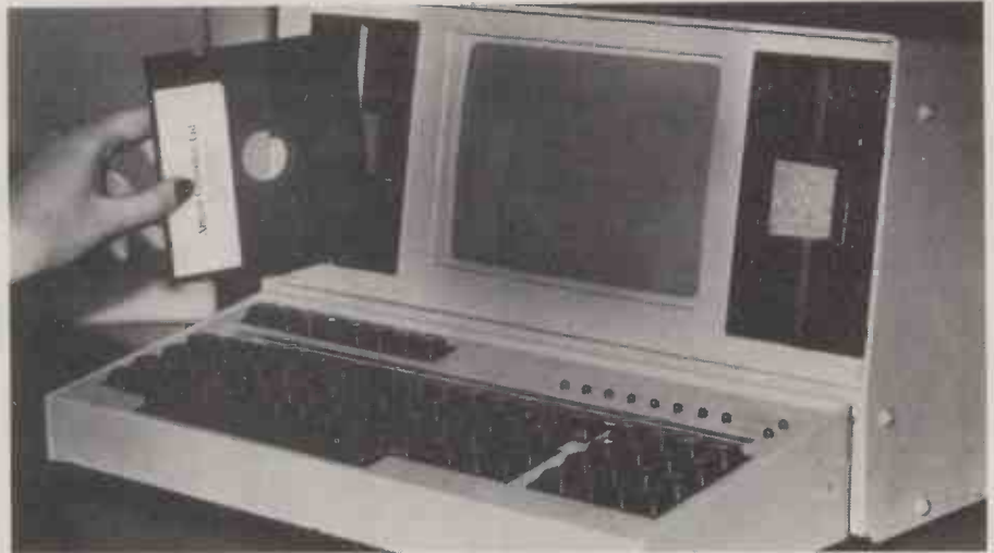
The top row of the keyboard has eight user-definable keys, useful for process control, and eight lights connected in parallel with the disc access port. These lights can be user defined, with labels put next to them to signal specific conditions to an operator.
